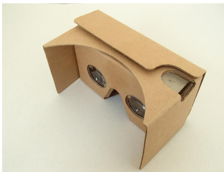
Figure 1: Google cardboard 3D glasses contain two optical lenses and a space for the smartphone at the front. The glasses have an action button to increase the interactive experience the user has with the virtual environment.
