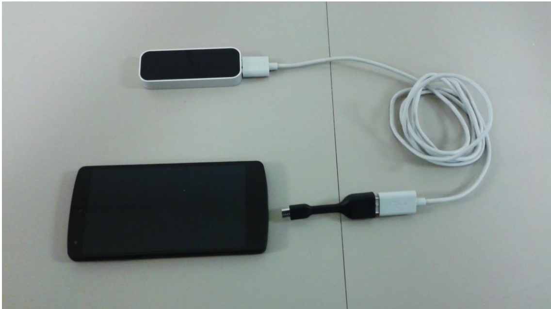
Figure 21: The setup of the smartphone with the LM controller. The LM uses a USB connector, so a USB to micro USB converter was needed to connect the LM directly to the Nexus 5.
