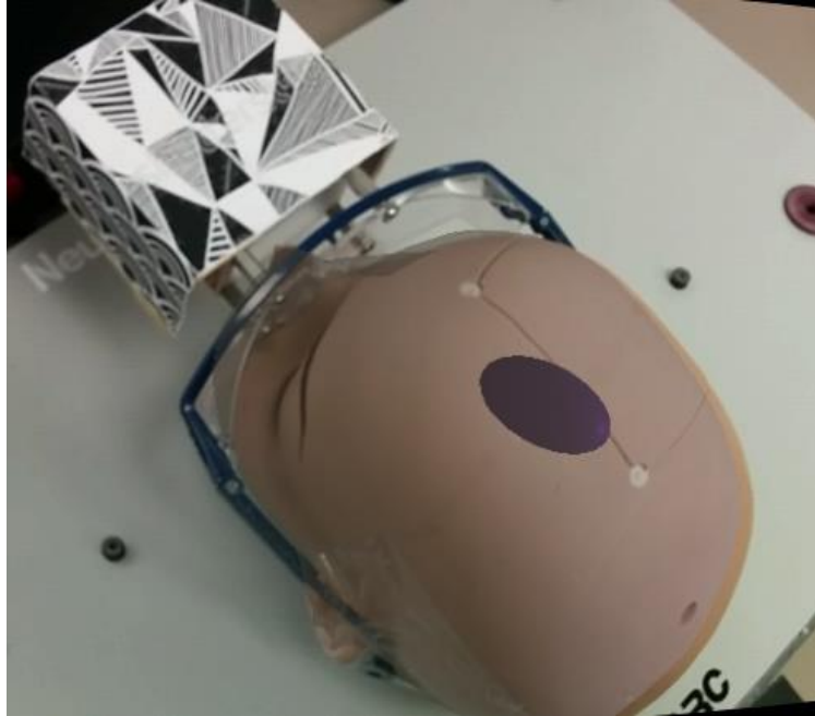
Figure 48: The transparent virtual head overlaid with the physical head.
